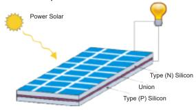
Photovoltaic solar energy which can be used in the generation of electricity through the use of photovoltaic solar panels (PV) that convert solar radiation into electricity, making it applicable to multiple activities of life.
